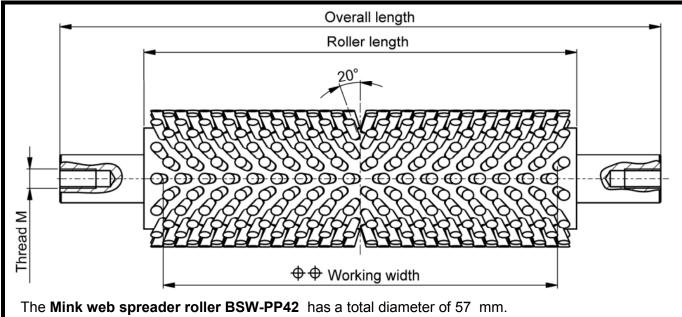
The steel shaft fully mounted on ball bearings has a diameter of 20 mm h9.
