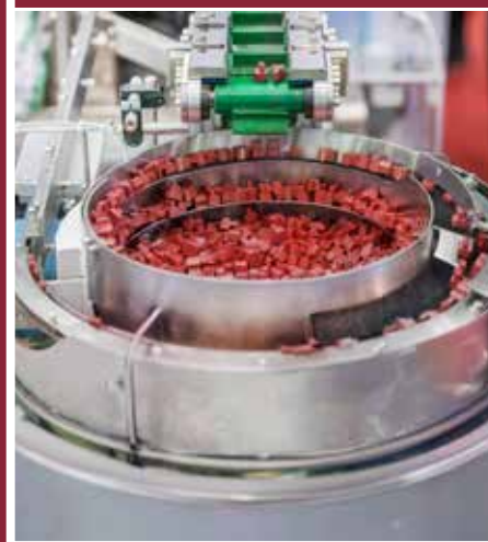
Mink Slide-Brush® in una mangiatoia a ciotola Mink Slide-Brush® in a spiral conveyor
