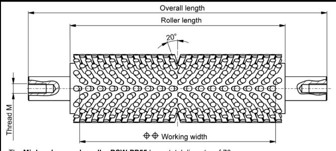
The **Mink web spreader roller BSW-PP55** has a total diameter of 70 mm.
