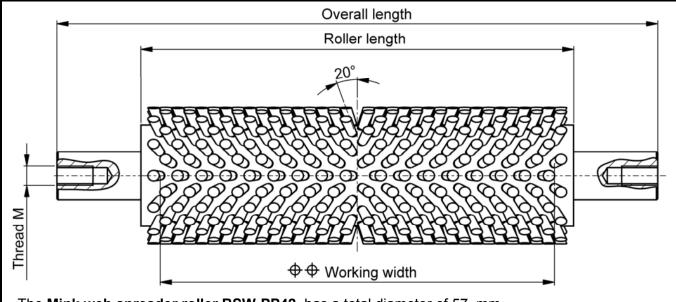
The Mink web spreader roller BSW-PP42 has a total diameter of 57 mm.
